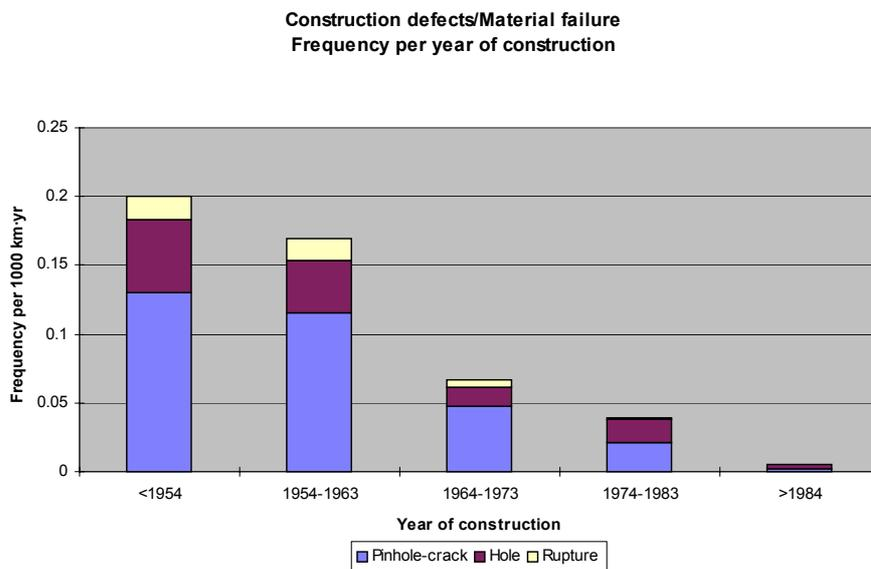
**Figure 12.** Failure frequency due to material and construction defects per year of construction
