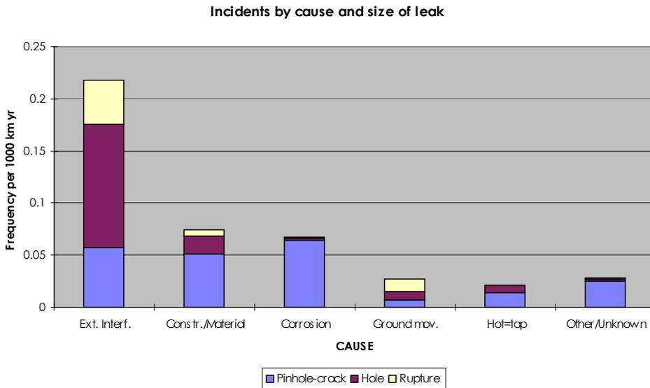
**Figure 8.** Incidents by cause and size of leak
